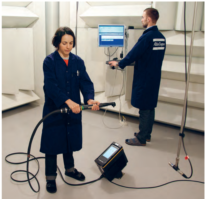
Atlas Copco has a well equipped laboratory for measuring tool noise and vibration emissions. It contains advanced vibration measurement tools, a state-of-the-art acoustics laboratory and dedicated computer software for analysing measurement and test results.
